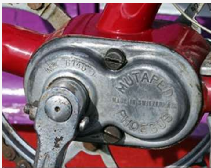
The 1937 bracket used 2 bolts; from 1941 on they used 5 bolts (left one is missing)
