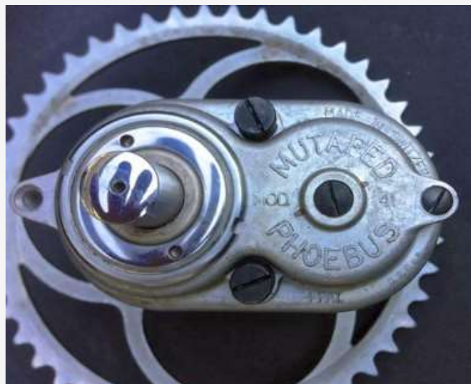
The 1937 bracket used 2 bolts; from 1941 on they used 5 bolts (left one is missing)
