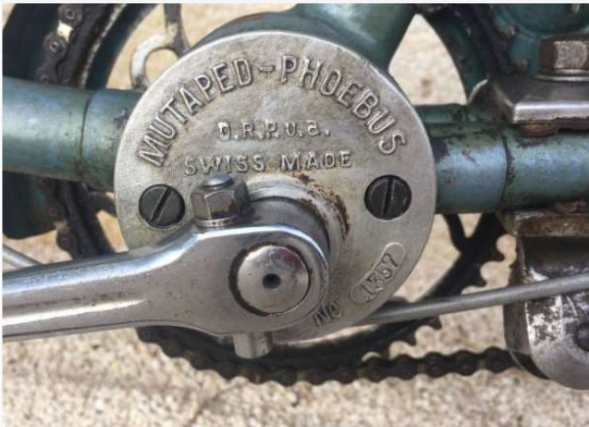
The 2-speed from 1935 had a round bottombracket.
